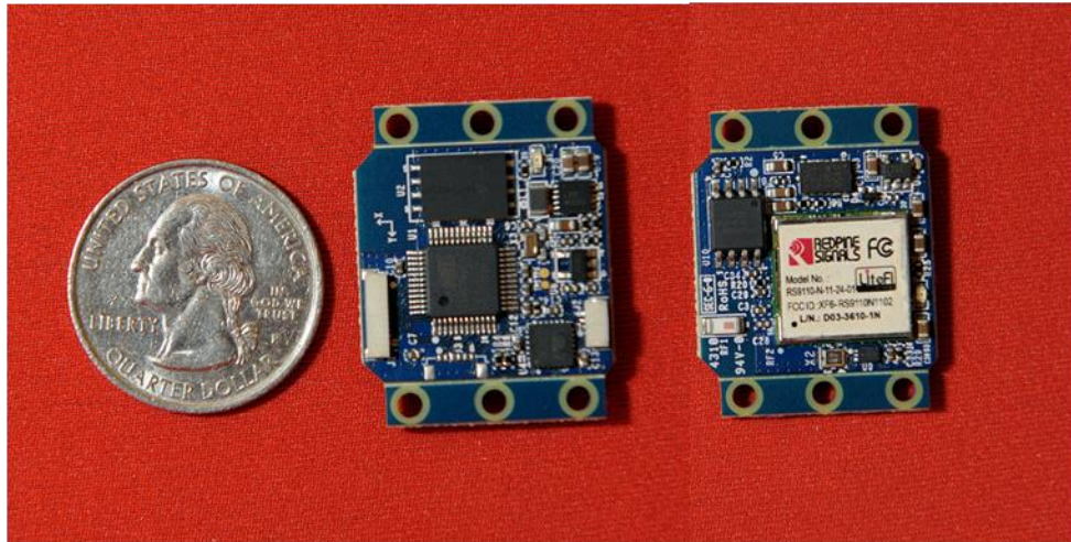
Figure 2.1: Highly miniaturized wireless IMU design used in this study was approximately the size of a quarter. The IMU provides three-axis sensing of acceleration and angular velocity with wireless data transmission to a host computer.
